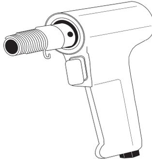
1. Uses reciprocating motion to provide rapid impact force, much like a rapid series of short hammer blows
