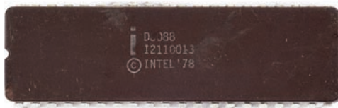
• Figure 5.20 The dual inline pin package of the Intel 8088
