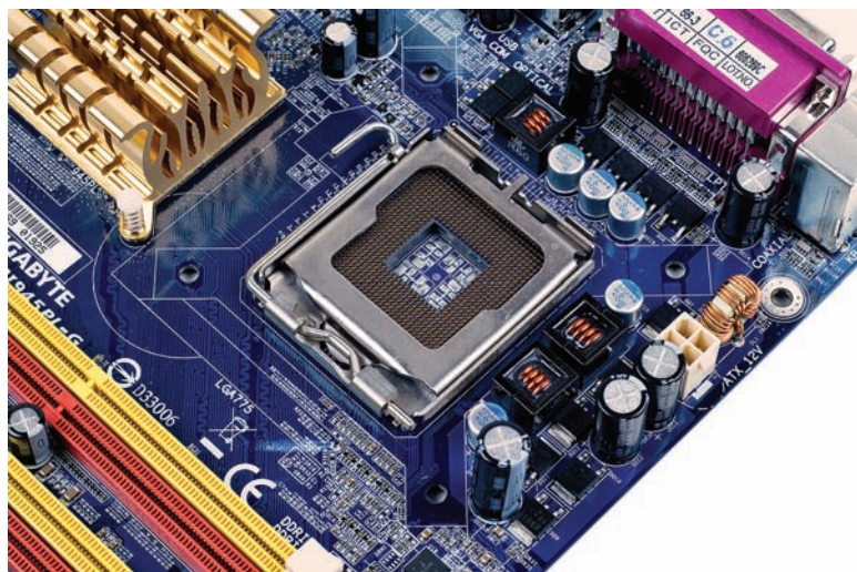
• Figure 5.24 ZIF socket with cage over the top
