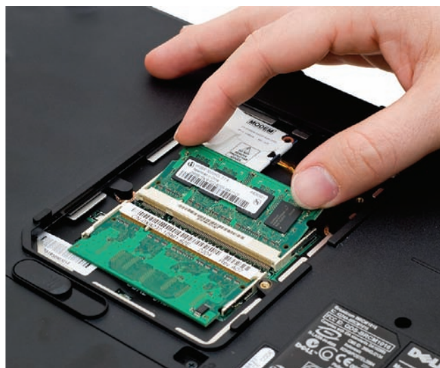
• Figure 6.33 Snapping in an SO-DIMM
