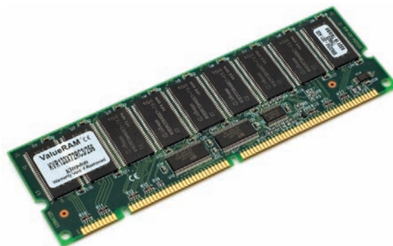
• Figure 6.21 Buffered DRAM
