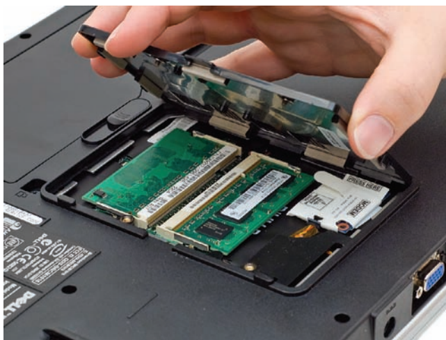
• Figure 6.32 A RAM access panel on a laptop
