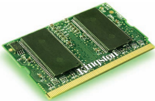
• Figure 6.14 172-pin DDR SDRAM micro-DIMM (photo courtesy of Kingston/Joint Harvest)
