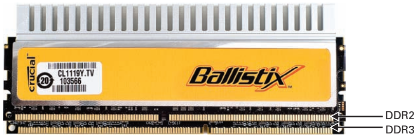
• Figure 6.17 DDR2 DIMM on top of a DDR3 DIMM
