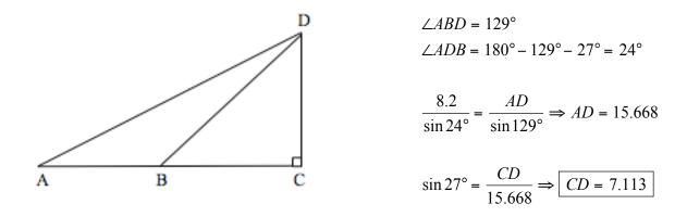
3. In the figure above find segment CD if  $\angle A = 27^{\circ}$ ,  $\angle B = 51^{\circ}$  and  $\overline{AB} = 8.2$  miles
